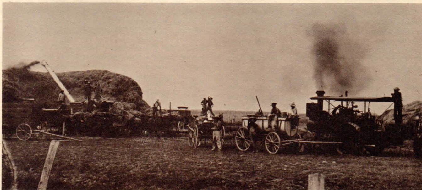
A steam threshing machine, used for wheat and oats, could thresh between 400 and 500 bushels per day if a breakdown did not occur. (Tippecanoe County Historical Association archives)
